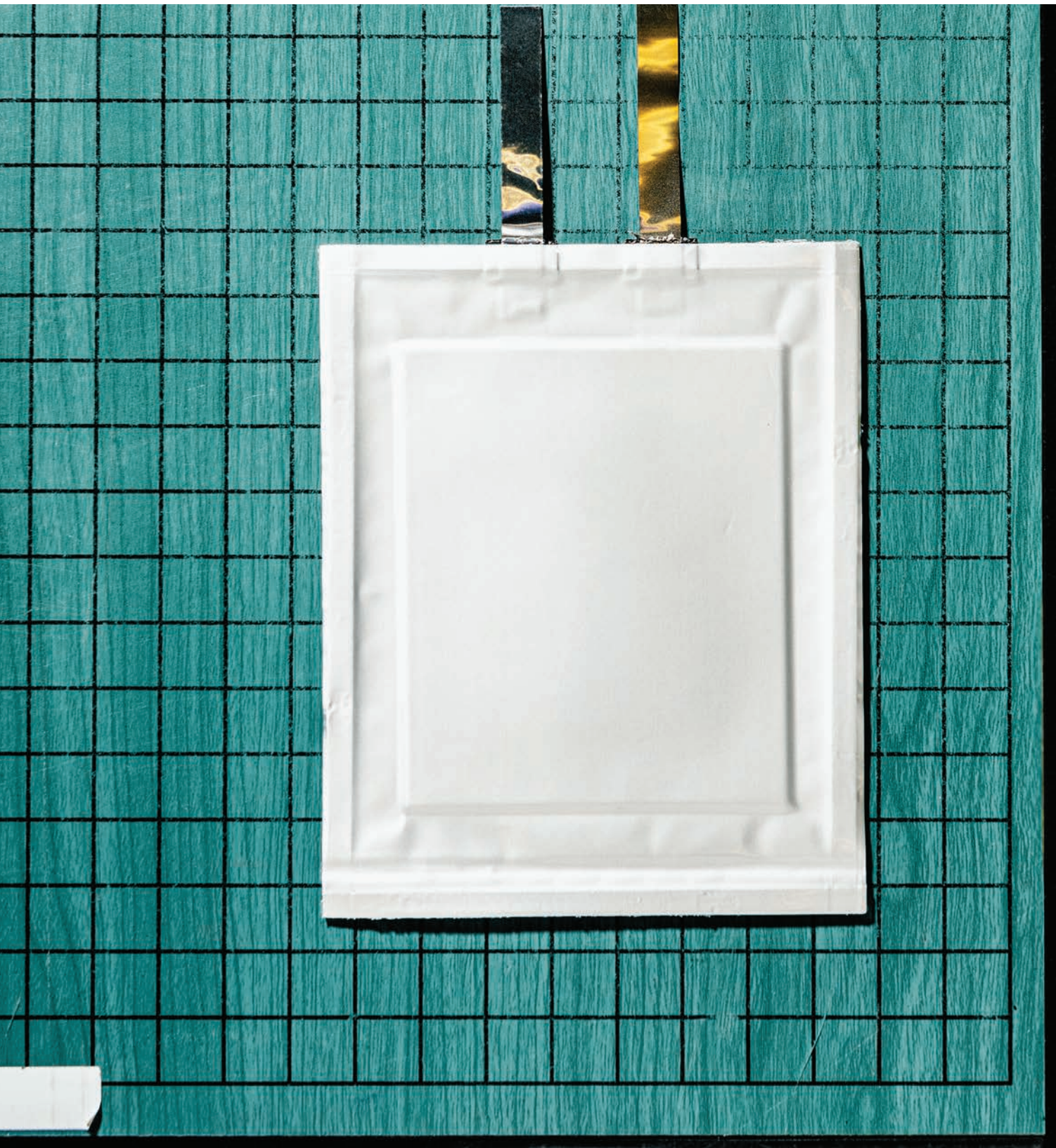
QuantumScape's prototype cell features a solid version of the usually liquid electrolyte.
